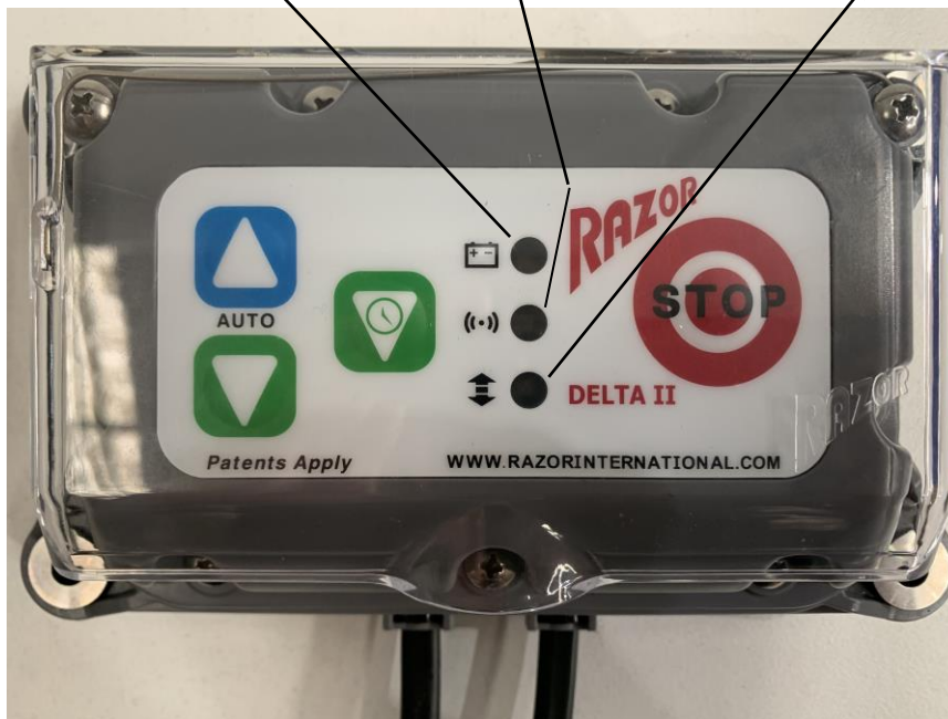
Battery Light Comms Light Status Light
