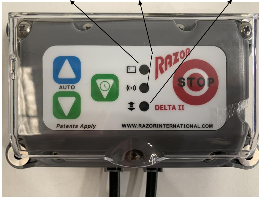
Battery Light Comms Light Status Light
